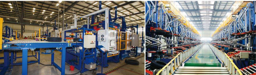
●Automatic tiered warehouse facility curing moulds | ●Extruder line From Germany Troester
